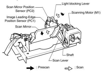
The Image Leading-Edge Position Sensor (PC1) and Scan Mirror Position Sensor (PC2) detect the cutouts in the light blocking lever.
